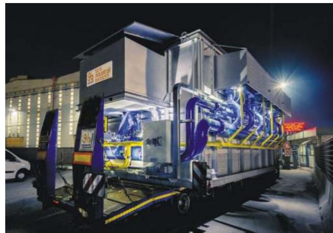
The prefabrication concept, applied to all the furnaces and peculiar to **bendotti**, gives unique advantages during the erection on site such as reduced erection time and consequently lower costs and earlier production, with no need either for refractory specialists or for tools for refractory on-site installation.
